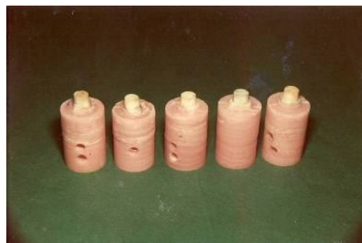
Fig. 1 Prepared teeth samples embedded into cylindrical shape blocks
