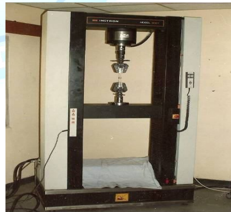
Fig. 5 Performing retention test using Instron tensile testing machine
